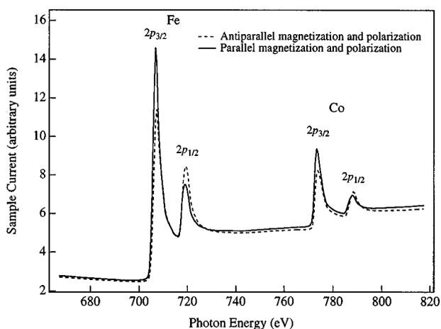
FIG. 10. An example of MXCD absorption is shown here. The 5 ML ( $\text{Fe}_3\text{Co}_1$ )Cu(001) sample was magnetized in-plane. The degree of circular polarization was approximately 70%. This lower-than-usual value was chosen for ease of operation and enhanced counting rates. Corrections for non-ideal polarization (<100%) can be made following Ref. 8. Regardless, strong dichroisms are easily observable here.
