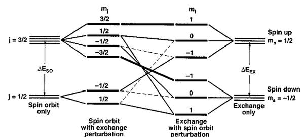
Fig. 9. The effect of spin orbit and exchange splitting upon a p core level is illustrated here. Two perturbative approaches are shown: large spin orbit and small exchange splitting (left) and small spin orbit and large exchange splitting (right). The Ni 3p would fall to the left while the Fe 3p is near the center, where spin orbit and exchange effects are nearly equal and a non-perturbative approach is required. State mixing is indicated by dashed and solid lines.
