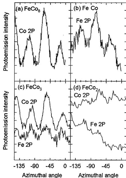
FIG. 5. XPD azimuthal scans are shown here, for a series of FeCo alloy overlayers, with the energy set to the core levels of either Co or Fe. The polar angle is  $45^\circ$ : the diffraction peaks demonstrate the degree to which the overlayer atoms are occupying ordered lattice sites.
