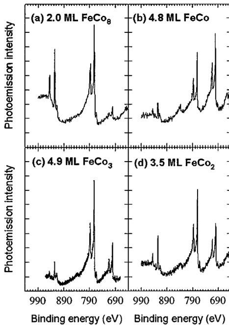
FIG. 4. XPS analysis of various  $\text{Fe}(1-x)\text{Co}(x)$  alloy overlayers on  $\text{Cu}(001)$ . Spectral structure includes the  $\text{Fe } 2p$  ( $B^F=707, 720$  eV),  $\text{Co } 2p$  ( $B^F=778, 793$  eV) and  $\text{Cu } 2p$  ( $B^F=932, 952$  eV). The sample in (c) may be slightly Fe rich at the interface; this effect was not included in the concentration estimate.
