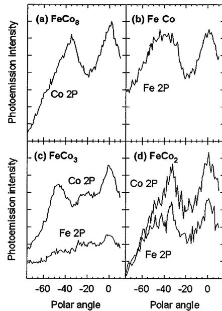
FIG. 6. XPD polar scans are plotted in this figure. The azimuth is set on a peak and the polar angle is scanned. For a, b, and d, the plane of rotation is a  $\{110\}$  plane. For c, it is a  $\{100\}$  plane.
