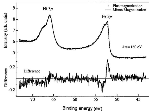
Fig. 8. Photoelectron spectra of 2 ML (Fe[1]Ni[4])Cu(001), taken using a photon energy of 160 eV. Again, a difference spectrum is also shown, as a measure of the MXLD effect.
