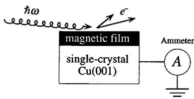
FIG. 2. Shown here is a schematic representation of the MXCD absorption experiment. A total yield method has been used. The picoammeter (A) monitors the grounding current, giving a measure of the absorption in an ultrathin film. It is necessary to align and antialign the magnetization and helicity or circular polarization, hence grazing incidence ( $15^\circ$ ) is used with in-plane magnetized samples (see Ref. 8).
