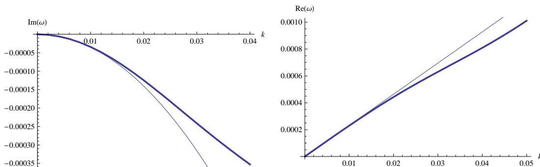
**Figure 5.** Fits of the real and imaginary part of the hydrodynamic modes in the broken phase to the lowest order approximation  $\omega = v_s k - i\Gamma_s k^2$ . The left figure shows the real part and the right one the imaginary part. The thick lines are the numerical results and the thin lines are the linear and quadratic fits. The fit is done for a temperature just below the critical one where the range of the approximation is rather small.
