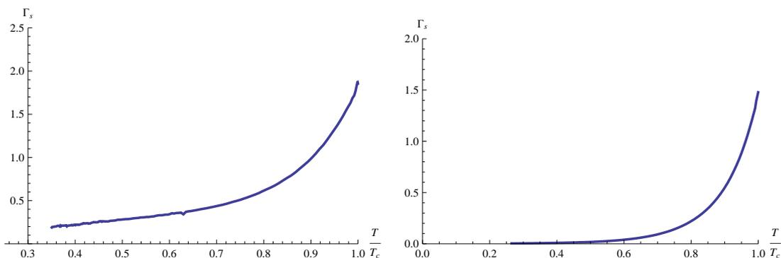
**Figure 7.** The plots show the attenuation constants of second sound as extracted from the location of the lowest quasinormal mode in the broken phase. The left figure is for the  $O_1$  theory and the right one for the  $O_2$  theory. Again it can be noticed that the  $O_1$  theory is numerically more challenging at low temperatures.
