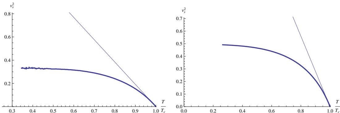
**Figure 6.** The plots show the squares of the speed of sound as extracted from the location of the lowest quasinormal mode in the broken phase. The left figure is for the  $O_1$  theory and the right one for the  $O_2$  theory. We also indicate the linear behavior close to  $T_c$ . As can be seen the numerics for the  $O_1$  theory becomes somewhat unstable for low temperatures.
