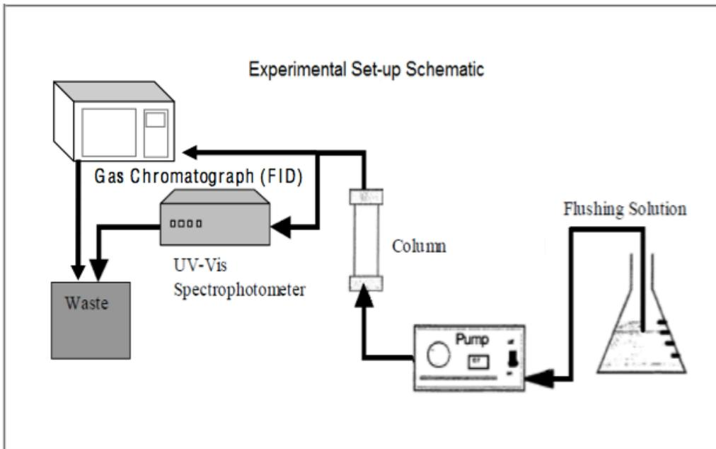
**Figure 1.** Schematic of Experimental Setup (adapted from [Burke, 2011](#)).
