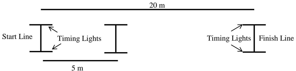
Figure 2.3 Straight-Line Sprint Test set-up.
