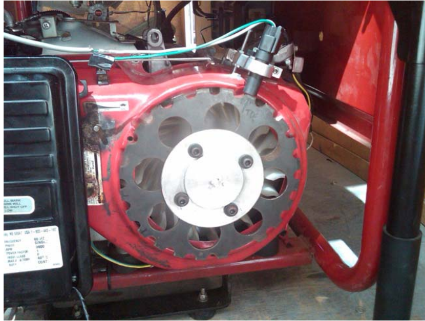
Figure 2.1: Crank Position Sensor and 24 Tooth Crank Wheel.
